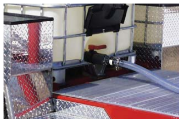
Direct Tank Hook-Up To Nozzle
