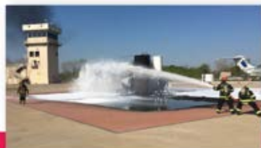
Firefighter training with the "roll on" and "rain down" application technique at .13 gpm/ft 2 using standard equipment with Avid F3 Green
