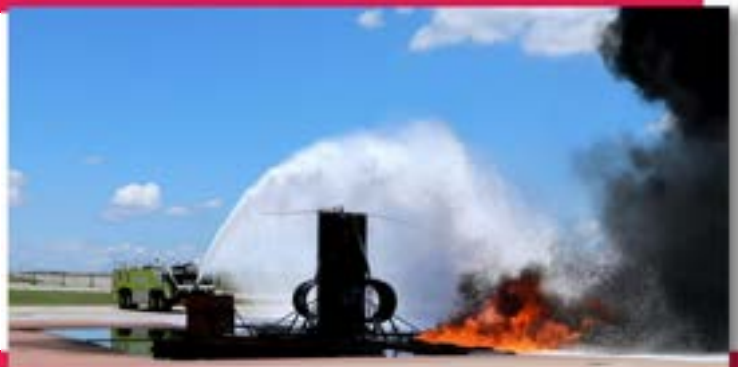
National Foam Avio F3 Green ICAO level "C" firefighting foam live fire testing at DFW
