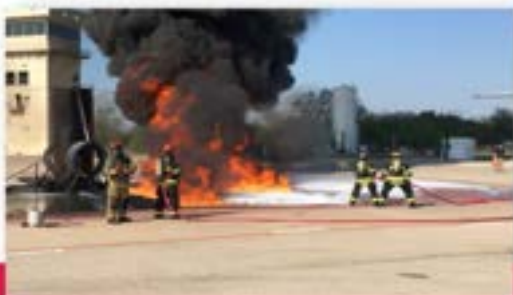
Firefighter training with the "roll on" and "rain down" application technique at .13 gpm/ft 2 using standard equipment with Avid F3 Green
