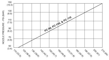
STRAIGHT STREAM RANGE IN STILL AIR - FEET (METERS) Range is with nozzle elevated 22.5° and nozzle inlet 3-6 ft (1-2 m) above ground level
