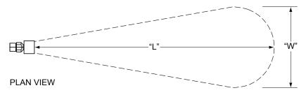
Note: Spray pattern based on nozzle mounted 36" (914.4 mm) above grade.
