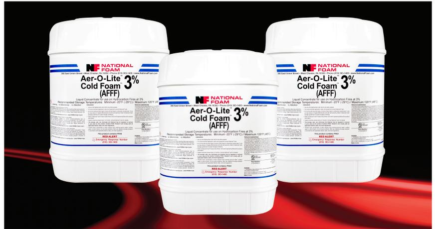
AFFF foam concentrates are designed for rapid fire knockdown by producing a thin aqueous film which spreads across the surface of the fuel, separating the fuel from oxygen. This is accomplished by allowing the foam solution to quickly drain from the foam bubble which in turn, affects long term sealability and burnback resistance.
